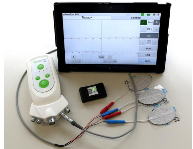
Fig 4. Autonomous Feedback-Controlled Drop Foot Stimulator consists of a) RehaMovePro, b) wireless inertial sensor, c) tablet computer with the graphical user interface.
