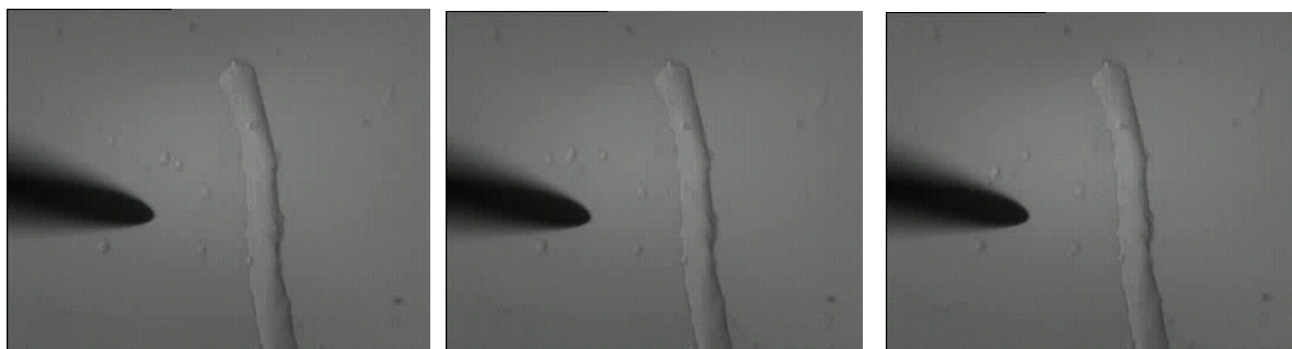
Fig. 5 Migration of particles inside the electrical field during stimulation. A group of three particles are visible close to the tip of the electrode on the left side and a single fiber on the right side. The relative changes in position are detectable by eye comparing the three images taken at subsequent times.
